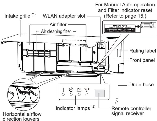
\*1) Before starting operation, make sure that the intake grille is closed completely. Incomplete closing may affect the proper function or performance of the product.
