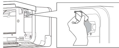
4. Remove the WLAN adapter from the connection slot of the indoor unit in the direction as shown in the figure.
