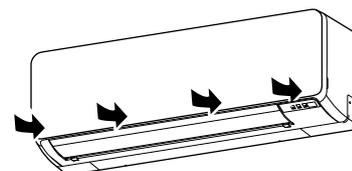
**NOTES:** If dirt accumulates on the air filter, airflow will be reduced, operating efficiency will lower, and the noise will increase.
