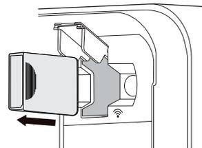
5. Close the WLAN adapter cover and the intake grille.
